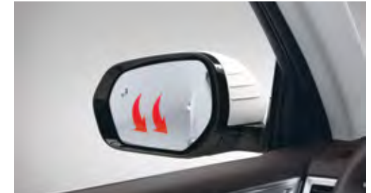
Reverse inter-locked auto-down outside mirror
